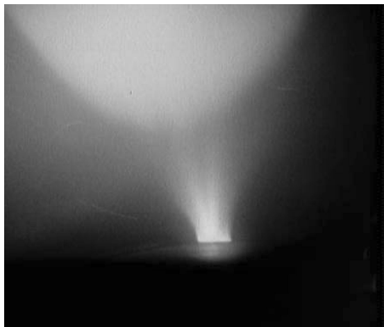
Fig. 1 Exhaust plume of an orbiter primary reaction control system thruster.
